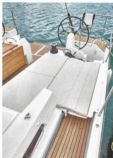
Above: the cockpit coamings fold out to make sunbed loungers
