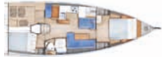
Version A Forward Owner's cabin, 1 aft cabin / 1 head Sink-dressing in forward cabin, optional
